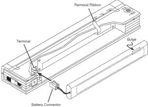
Figure 11. Pushing the battery connector into the terminal
